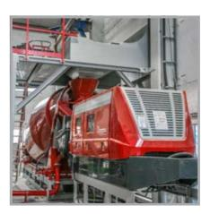
The buffer storage can be placed directly under the mixing plant or can be filled via an existing bucket conveyor.
