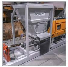
For small precast parts or small mixing plants a hopper extension is enough to guarantee the continuous supply of the concrete pump with concrete.
